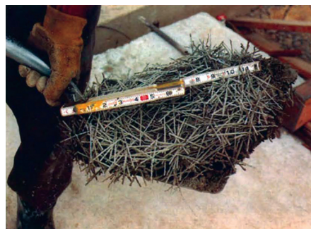
Fig. 7 – Steel fibers 2.5 in. long created tensile forces to hold the slab in compression as Type K cement expanded.
