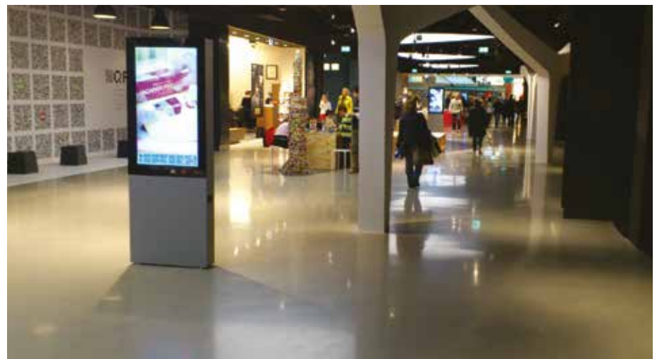
KÖLN ARCADEN SHOPPING MALL: Required replacing an 18,300-square-foot area of existing stone tile floor. Rapid Set TRU Self-Leveling was chosen to resurface the floor because it provides a high quality, decorative surface in a short time frame.
