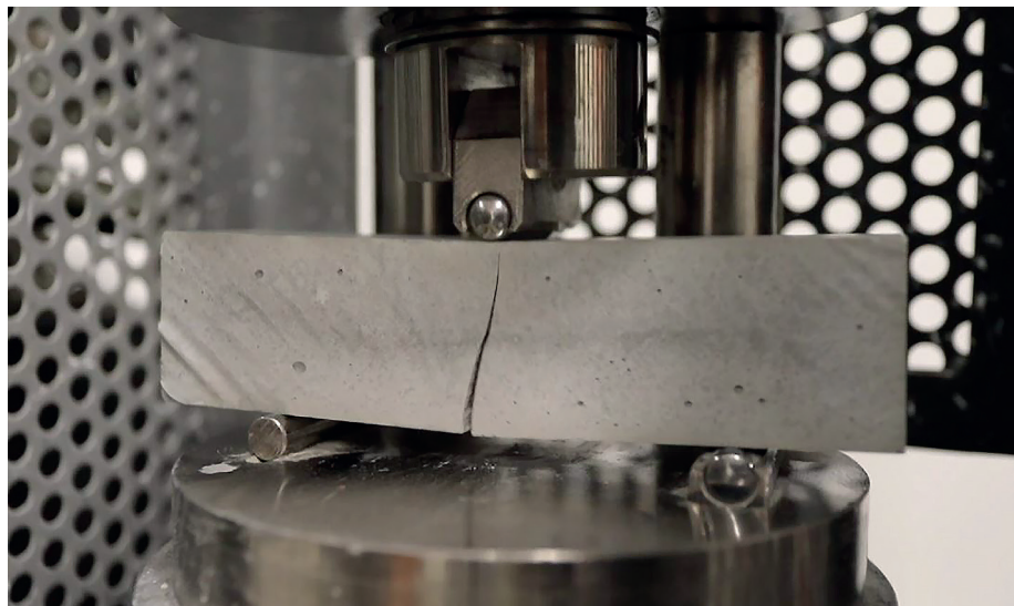
The downward force from the top causes the bottom of the prism to fail in tension during this ASTM C348 Test performed at the CTS laboratory.
