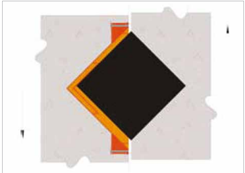
Fig. 5 – The diamond plate dowel system allows for differential shrinkage in adjacent slab placements, allowing the joint to open freely and provide total load transfer.
