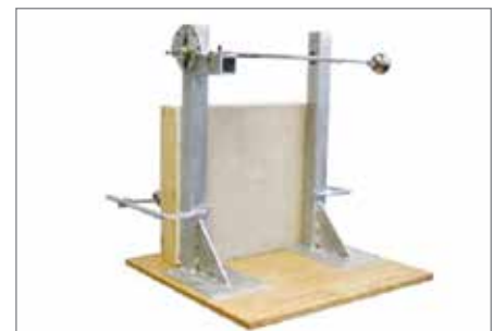
Fig 6 - This impact tester uses a steel ball on a pivot to measure the amount of impact energy absorbed by a wallcovering material. Rapid-setting CAS plaster tested to about twice the impact resistance of portland cement plaster.
