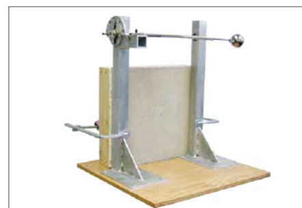
Fig 6 - This impact tester uses a steel ball on a pivot to measure the amount of impact energy absorbed by a wallcovering material. Rapid-setting CAS plaster tested to about twice the impact resistance of portland cement plaster.
