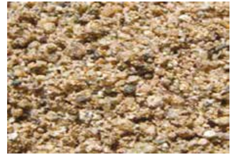
Fig 4 - Plaster sand must have certain physical characteristics of grain shape. Where there is any doubt, premixed bagged plaster products may be specified. Photo © Steven H. Miller
