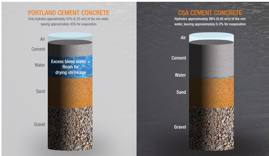
Excess bleed water in portland cement designs leaves room for drying shrinkage as voids and capillary channels are created upon egress of the excess mix water. CSA cement's hydration mechanism consumes H_2O molecules in the creation of ettringite crystals, effectively eliminating excess bleed water and preventing dryage shrinkage.
