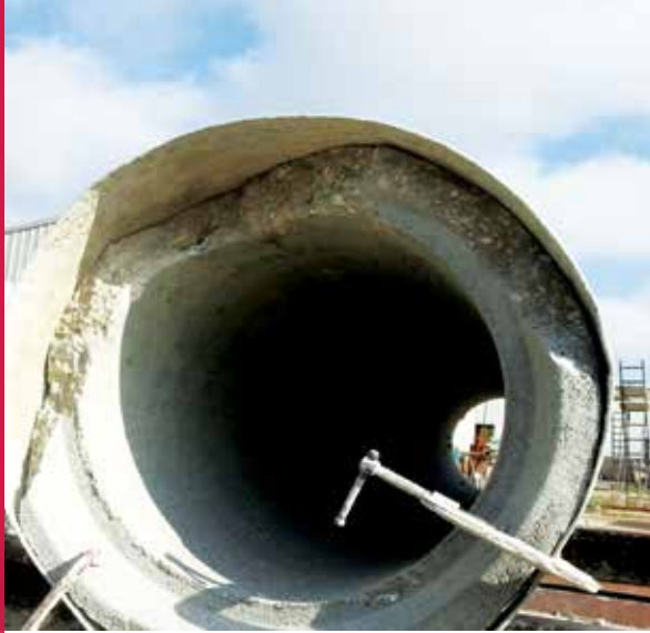
Rapid Set® Mortar Mix precast concrete pipe (Houston, TX)
